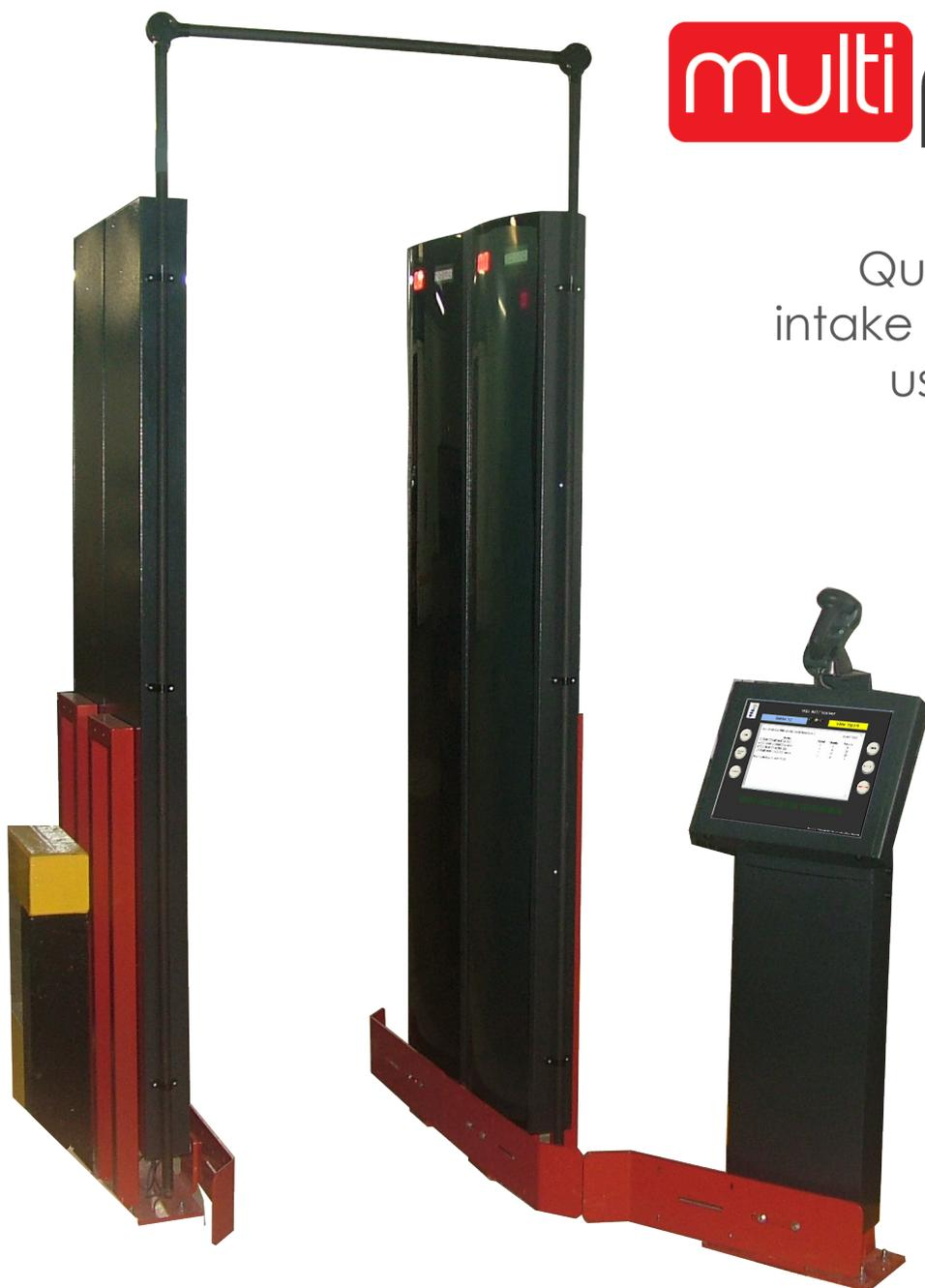
Our multiportal<sup>TM</sup> 400 offers flexibility and resilience for both Marks and Spencer RFID tag writing and despatch processes. The multiportal<sup>TM</sup> 400 configuration is made up of four independent columns that incorporate the antennas, these are connected to an ultra slim touch screen control console that holds the RFID reader.
