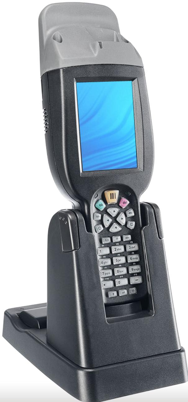
The multi<sup>TM</sup>terminal 100 is designed to perform several functions including; laser scanning a tray label, reading an individual tray tag, writing an individual tray tag and verifying an individual tray tag.
